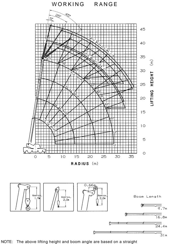
(unladen) boom, and allowance should be made for boom deflection obtained under laden conditions. The above working range is shown on condition with outriggers fully(6.3m) extended.
